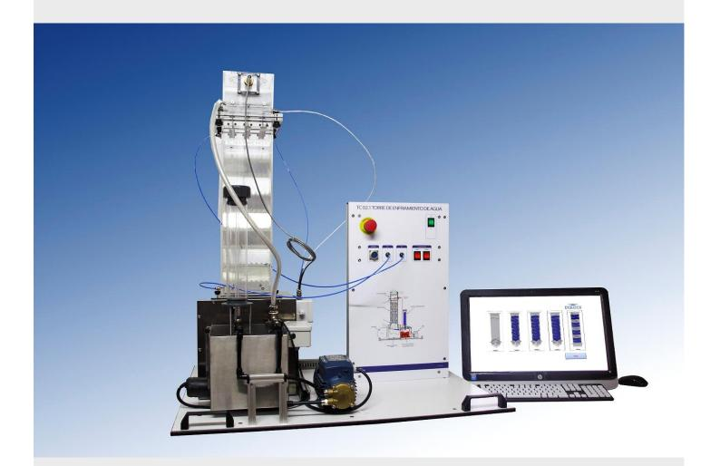
The TC 02.1 unit operates a standard cooling method, used in the industrial sector. This method involves cooling hot water to environment temperature.
