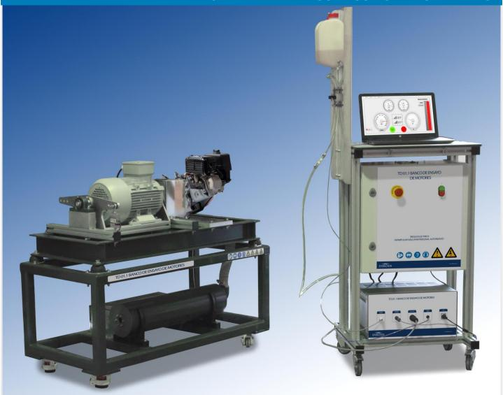
The TD 01.1 equipment, has been designed for the study and understanding of the behavior of a gasoline four-stroke combustion engine.
