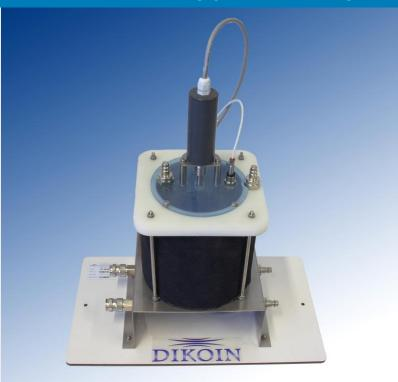
Optional Accessory: TC 01.5 - DOUBLE JACKETED VESSEL AND COIL HEAT EXCHANGER
