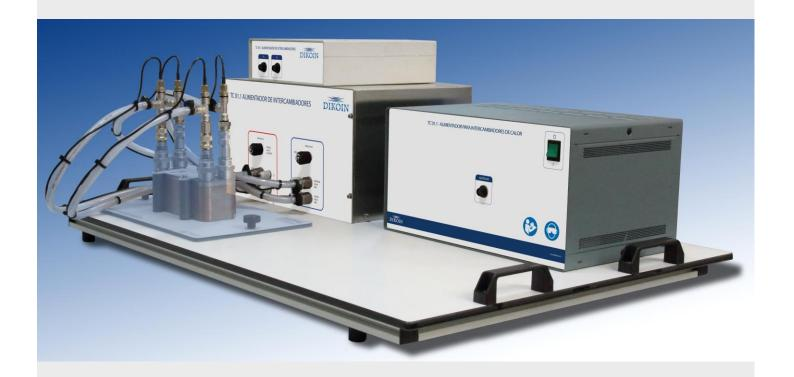
The TC 01.1 equipment is the core of the whole heat exchanger. TC 01.1 is the module that provides hot and cold water to the heat exchangers, in addition to measuring the temperatures and flow rates for each device.
