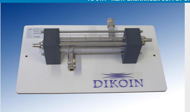
Optional Accessory: TC 01.3 - SHELL TUBE HEAT EXCHANGER
