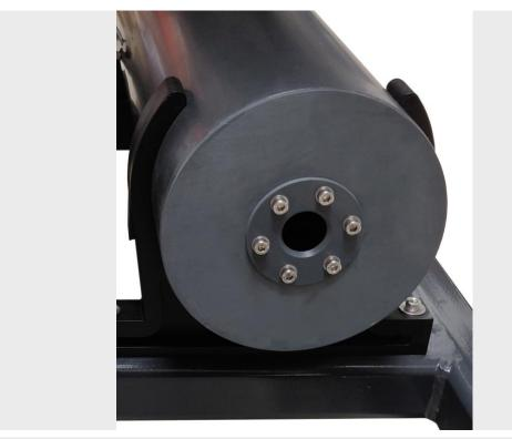
The system has a device for measuring the volume of air sucked by the engine, so that calculations can be made corresponding to the air-fuel ratio, etc.
