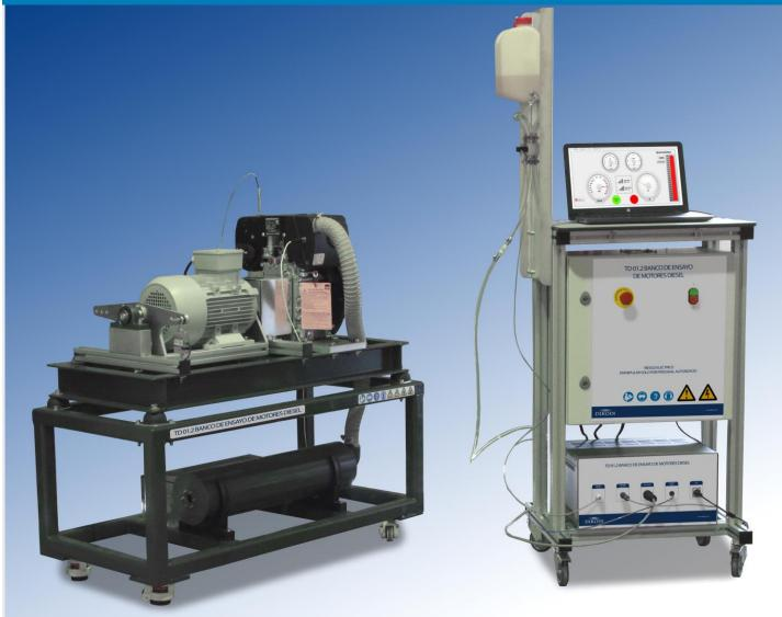
Equipment designed for the study and understanding of the behavior of a four-stroke single cylinder diesel combustion engine.
