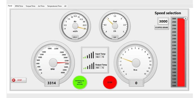
The equipment includes a PC with the equipment management software. In which, the parameters of all control points of the equipment are shown, and the data collection is allowed in automatic or manual mode.
