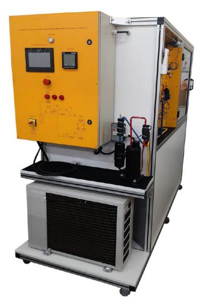
The bench for the Study of Energy Efficiency in HVAC (Air Conditioning) Systems was designed to allow the study measurement of electrical consumption, temperature gradients, possible failures and loss of performance in an air conditioning system that includes the reverse cycle. It allows to demonstrate in practice, the differences in the energy consumption and the energy efficiencies of the system, with the insertion of faults that commonly occur in climate-controlled environments.
