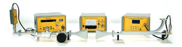
The trainer has been designed to introduce students to the microwave technology. It consists of a set of components, accessories and instruments and can be used as a laboratory test bench to experiment with the microwaves components as well as to study the aspects of wave propagation.
