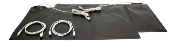
Timing mats are pressure sensitive switches designed to react to a person standing on the mat. They are digital switch-type sensors that have two states, ON and OFF. The mat is open (OFF), until someone stands on the mat and the switch is closed (ON).
