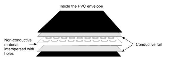
The Timing mats are designed for use on a flat even surface e.g. the floor. During use the Timing mat should be laid out and kept flat. The conductive foils must be protected from damage caused by the mat being distorted or pierced by sharp objects. If the surface under the mat is rough e.g. concrete, then protect by placing a smooth surface e.g. rubber mat under the Timing mat. The uppermost surface can be protected by covering the Mat with a conventional floor covering such as piece of carpet.
