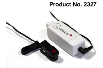
The Heart Rate sensor sensing clip (pleth) holds an infrared LED that shines a light through either a finger or ear lobe onto a light sensitive detector. As the amount of light transmitted varies with the flow of blood, the sensor can record either blood flow (heart waveform), or heart rate (beats per minute).
