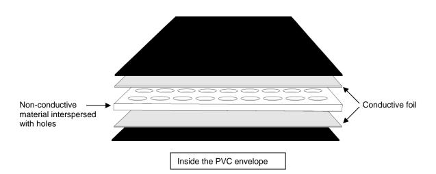
The Timing mats are designed for use on a flat even surface e.g. the floor. During use the Timing mat should be laid out and kept flat. The conductive foils must be protected from damage caused by the mat being distorted or pierced by sharp objects. If the surface under the mat is rough e.g. concrete, then protect by placing a smooth surface e.g. rubber mat under the Timing mat. The uppermost surface can be protected by covering the Mat with a conventional floor covering such as piece of carpet.
