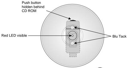
2. To record the speed of reaction you will need to enter the distance (in m) between the stimulus (the test subject seeing the LED light up) and the response (the test subject pressing the switch) i.e. use a fabric tape to measure the length from the subjects eye level, down the neck, along the outstretched arm to the thumb tip.
