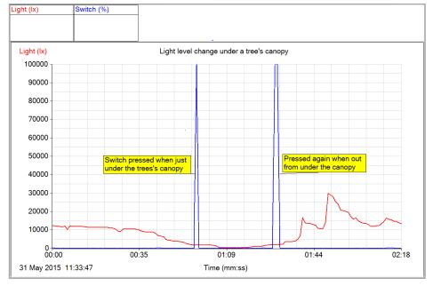
In this example a switch was used to mark two points (entry and exit) when walking with a Light Sensor under the canopy of a tree
