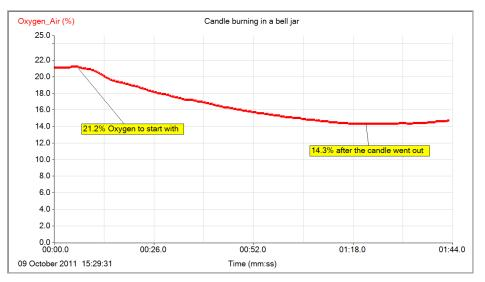
• Discovering the change in oxygen level during combustion - using a candle burning in a bell jar
