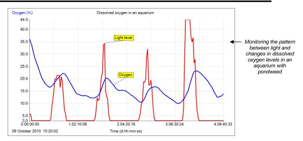
• Monitoring dissolved oxygen concentration resulting from photosynthesis and respiration in an aquarium containing plants and/or fish
