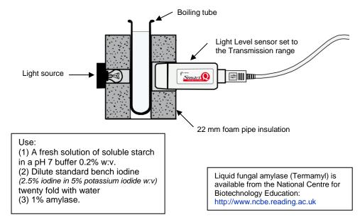
Assemble the apparatus as shown in the diagram and turn the light source on.
