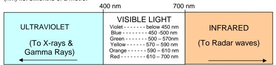
The Light Sensor utilises the photometric system of measurement that defines light in terms of how it is perceived by the human eye. The eye's sensitivity is dependent on the wavelength or colour of the light. Peak sensitivity occurs in the green part of the visible spectrum while the eye's response to infrared or ultraviolet is zero.
