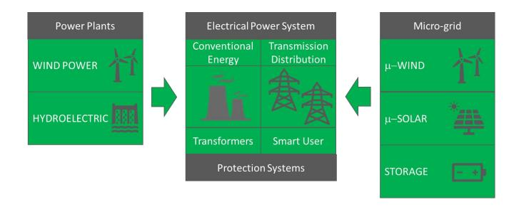
The core of the laboratory is a simplified scaled-down model of a power distribution system. Several power sources from different renewable energies are connected to the system on different points simulating a distributed power generation system. The energy can be added from the production side (high and mid voltage) or from the end-user side (microgrid).
