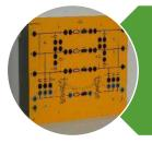
HV transmission lines of several lengths, busbar, and power switches simulate the power distribution and transmission system.
