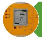
Synchronization relay to connect the generator to the grid.
