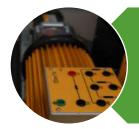
Synchronous generator that transforms the mechanical power into electricity.
