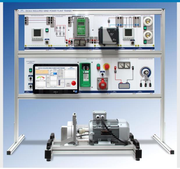
With this equipment, we emulated the behavior of a wind turbine in a practical and didactic way. An electric motor acts as the blades and bush of a wind turbine, dragging a three-phase synchronous generator of permanent magnets, which transforms the mechanical energy transmitted to the shaft into electrical energy at the output.
