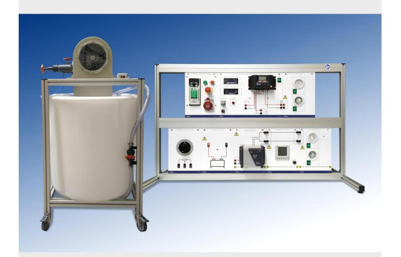
Trainer EN 05.1 has been designed as a small-scale hydropower plant and it is equipped with a Pelton turbine that provides full operation along with all the other accessories that complete a standard installation.
