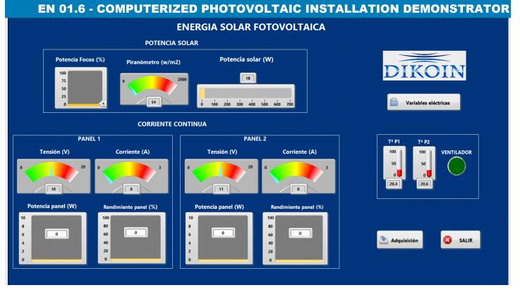
The equipment includes a PC with the equipment management software. In which, the parameters of all control points of the equipment are shown, and the data collection is allowed in automatic or manual mode.
