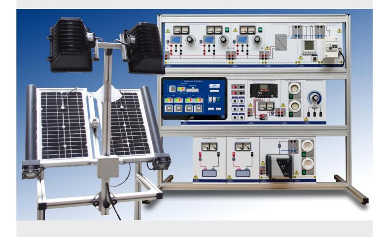
The EN 01.6 equipment scales a complete photovoltaic solar system. It has been designed with special emphasis on the didactic aspect of it, being able to observe at a glance all the components that a solar photovoltaic installation has and its arrangement. It allows the study of both, isolated photovoltaic solar energy installations and grid connection.
