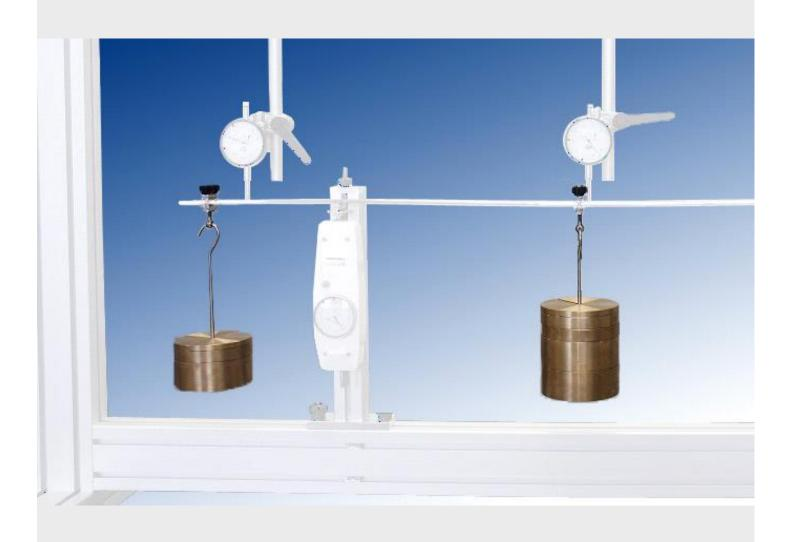
Weights system, with maximum load of 12 kg. Includes weights with different masses from 0,5 to 2,5 kg.
