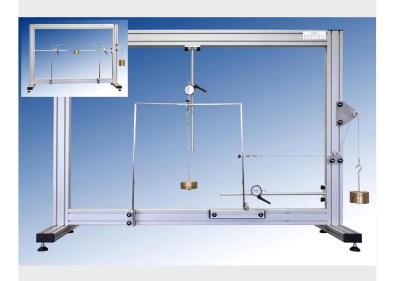
The objective of this equipment consists on the study of the deformation in the plane, of frame type structures under the action of solicitations. The equipment is supplied with a gantry in U and another with a "gable" roof.
