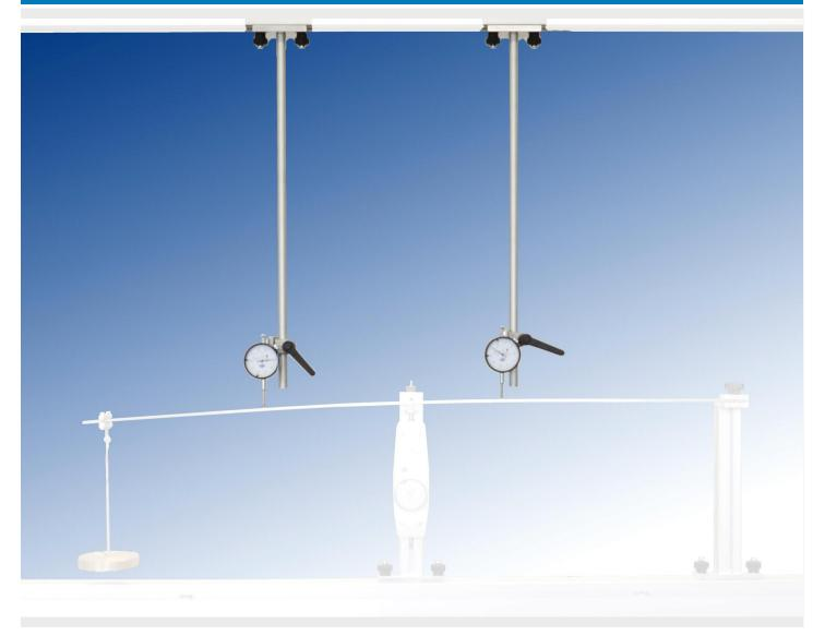
This is a displacement measurement system designed to be used with the ST series and to be mounted on a flat-structure frame. This accessory is composed by a pole (see top half of the image with 2 samples) that gets easily inserted into the frame of the ST 01.1 (not included), equipped with a gauge whose hand shows the range of displacement that has occurred from the starting point.
