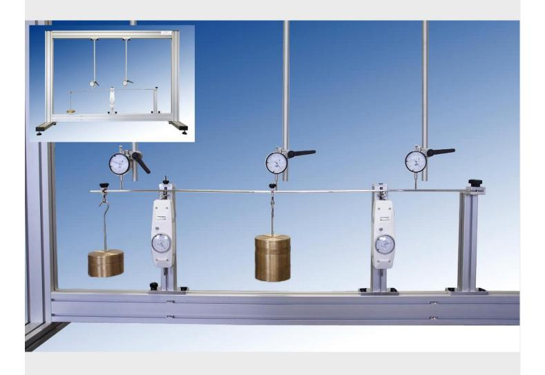
The objective of this equipment consists of the study of the deformation in the plane, of continuous beams under the action of loads.
