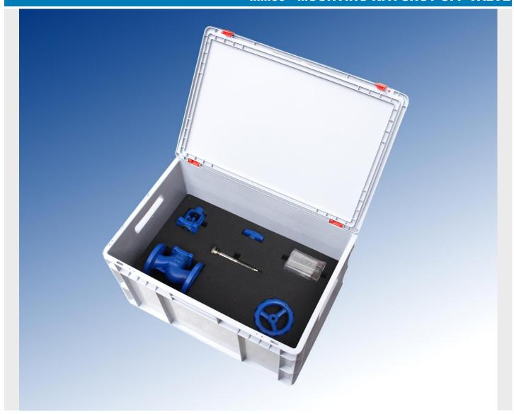
The mounting MM09 kit allows the assembly and disassembly of a shut-off valve. Thanks to the cutting it is possible to study each of the different components and their operation, for example, it is possible to observe how with this type of valves it is sought to avoid a sudden cut of the supply that originates the water hammer.
