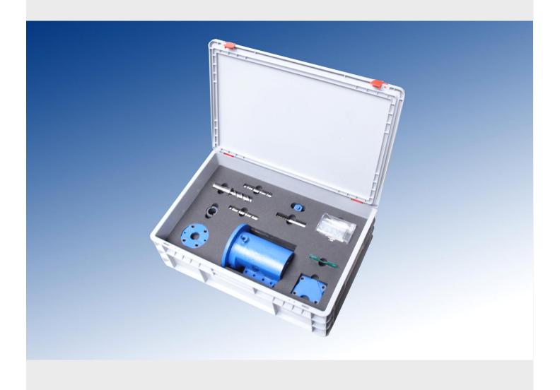
The assembly and maintenance MM04 kit allows the assembly and maintenance of a screw pump. These pumps allow the use of fluids other than water and therefore are usually used in lubrication with oils. Thanks to the cutting, the student learns all the components of the pump and its operation.
