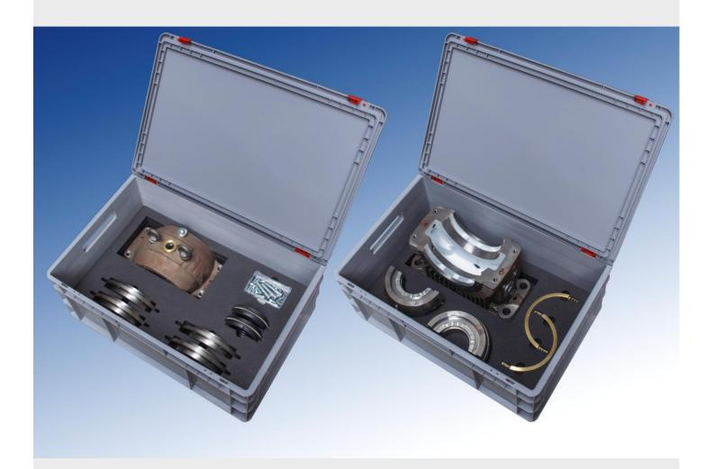
The MM08 mounting kit consists of a horizontally cut hydrodynamic bearing. In addition to the bearing, the equipment is supplied with an auxiliary shaft that facilitates the assembly and dismantling of the hydrodynamic slide bearing, thus the student learns all the components and their operation.
