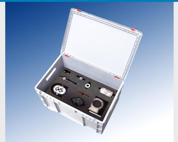
The assembly and maintenance MM07 kit allows the assembly and maintenance of a gear pump. In this type of pumps, the flow rate is proportional to the speed of rotation of the gears (rpm) and with them high pressures and service rates are reached. They are usually used with fluids of high viscosity and free of solid particles. Thanks to the cutting, the student learns all the components of the pump and its operation.
