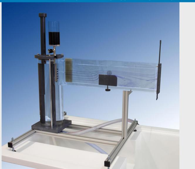
This equipment allows the study of the behavior of fluids in open channels and flow lines that form around different submerged objects.
