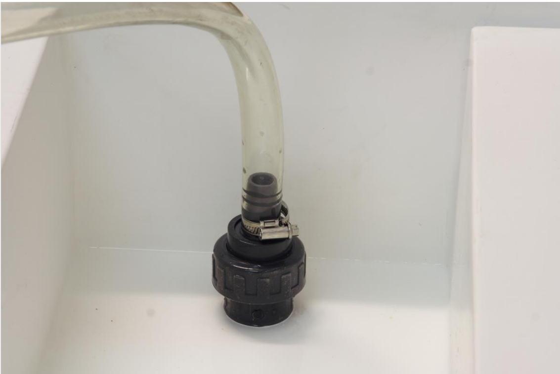
Easy connection of the equipment to the hydraulic bench.
