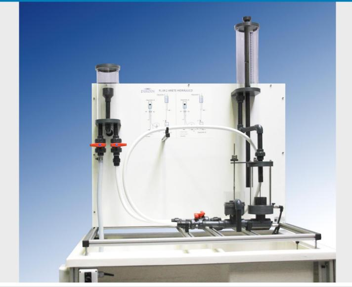
The FL09.2 is a equipment that aims to demonstrate and study the phenomenon known as water hammer, this phenomenon is the one that occurs due to the rapid closure of the passage of water through a pipe. The design of the equipment is made with special emphasis on the didactic field, so it is supplied with variable elements, to achieve a greater number of tests for a better understanding of the student.
