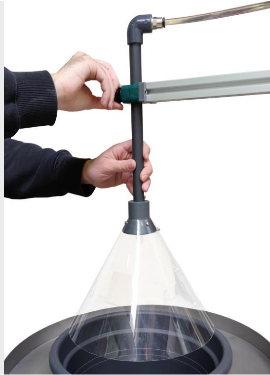
The equipment allows the height of the diffuser to be adjusted to position it correctly according to the flow rate used.
