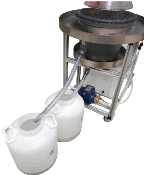
Two drums are supplied to collect and measure the amount of surface and groundwater runoff.
