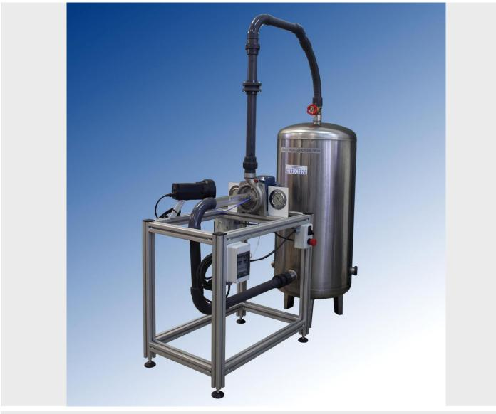
Cavitation is produced when a liquid that is being pumped loses pressure and matches the level at which vapour is generated at the same temperature the pump is operated. At that moment, liquid turns into vapour, giving rise to vapour locks or vacuum pockets that are pushed into other areas with a higher pressure. Very fast condensation takes place creating short-lived excess of pressure in very small places.
