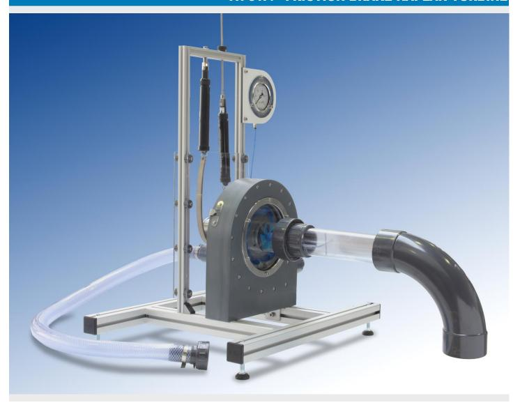
The TH 01.4 equipment simulates a small-scale installation with a Kaplan turbine.
