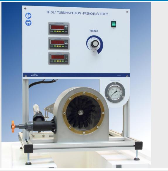
The TH 03.1 equipment simulates a small-scale installation with a Pelton turbine.
