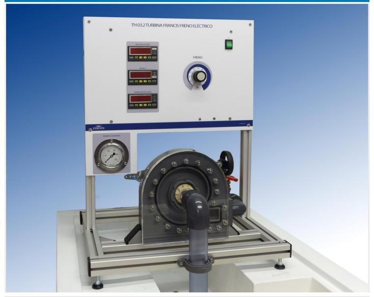
The TH 03.2 equipment simulates a small-scale installation with a Francis turbine or reaction.
