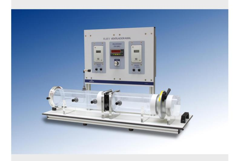
This equipment has been developed for the study of the characteristics of an axial fan, performing a range of practices and experiences.
