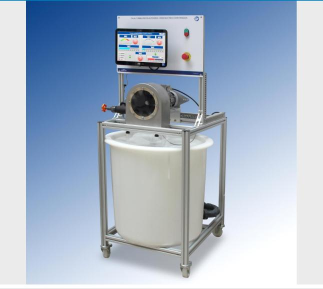
The TH 04.1 equipment simulates a small-scale installation with a Pelton turbine.
