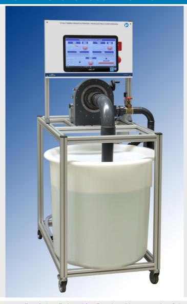
The TH 04.2 equipment simulates a small-scale installation with a Francis turbine or reaction. It is designed for the study and display both the behavior and the characteristics of a Francis turbine.
