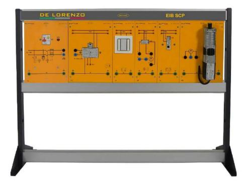
This laboratory is designed for the study of the shutter control plant and to allow the student a practical training, based on the performance of guided experiments. Industrial type components are educationally adapted by using a modular panel system to permit the step by step assembling from the simplest circuit to the most complex system.
