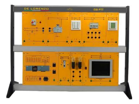
This laboratory is designed for the study of the plc, touch panel and time switch modules and to allow the student a practical training, based on the performance of guided experiments. Industrial type components are educationally adapted by using a modular panel system to permit the step by step assembling from the simplest circuit to the most complex system.
