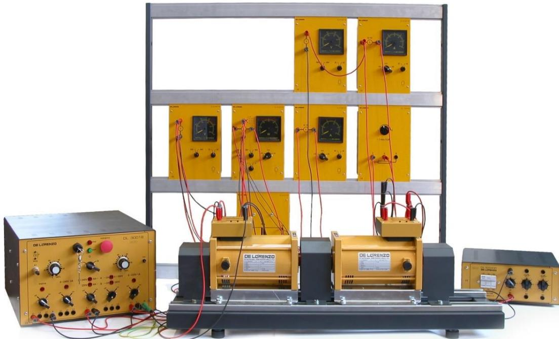
This system studies the topics related with the electric measurements. It has a modular structure and it consists of didactic panels installed on a vertical frame. The system is available in two versions: **DL 2109T** (study of electrical measurements) and **DL 2109TM** (study of electrical measurements with alternator)
