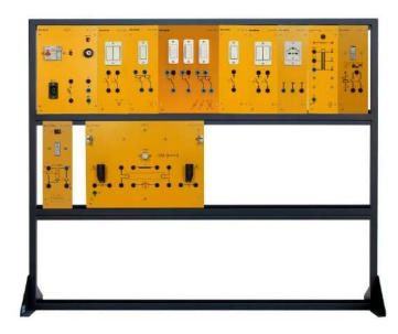
This system studies the topics related with the lighting plants in the electric civil installation. It has a modular structure and it consists of didactic panels installed on a vertical frame.
