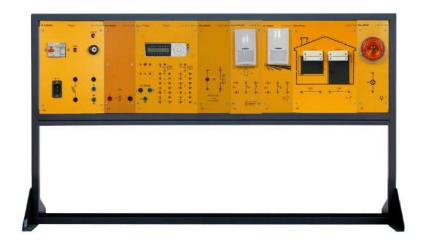
This system studies the topics related with a intruder alarm system in the electrical civil installation. It has a modular structure and it consists of didactic panels installed on a vertical frame.
