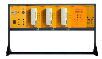
This system studies the topics related with the house phones. It has a modular structure and it consists of didactic panels installed on a vertical frame.
