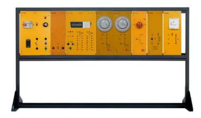
This system studies the topics related with a complete installation of a fire alarm system in the electrical civil installation. It has a modular structure and it consists of didactic panels installed on a vertical frame.
