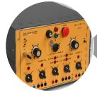
A three-phase power supply with fixed and variable outputs in AC and DC that provide the electrical power to the test bench and machines under study. The power supply includes all the protections needed to create a safe work environment for the student.
