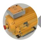
Electromagnetic brake for the characterizations of the motors with a load cell for accurate torque measurement.
