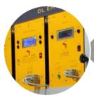
Multifunction digital modules to collect all the electrical parameters (voltage and current in AC and DC, RMS values, active, reactive and apparent power and frequency) and mechanical parameters (speed, torque) needed to characterize the machine under study.
