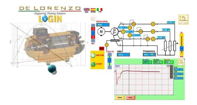
The automated test approach enables the student to monitor and control several variables of the electric machine under test in real-time, to easily observe their behaviour and interaction under several operating conditions such as load, no load, variable speed and torque, or different excitation values. The characteristic curves that can be obtained with the system provide accurate information to create a model of the machine, tune its controller and study the machine applications.
