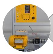
**Prime mover:** A squirrel cage three-phase asynchronous machine controlled by an inverter in four quadrant operation providing the mechanical power and torque necessary for the characterization of the machine under study.
