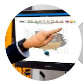
Data acquisition software for electric machines: performs the test automation and provides the user interface to execute the experiments. The SW developed in LabVIEW communicates with the acquisition devices via serial port using the Modbus protocol, reading electrical and mechanical data from instruments.
