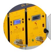
**Instruments:** collect mechanical data (speed, torque and temperature) as well as electrical data (AC and DC, Voltage, current and Power).
