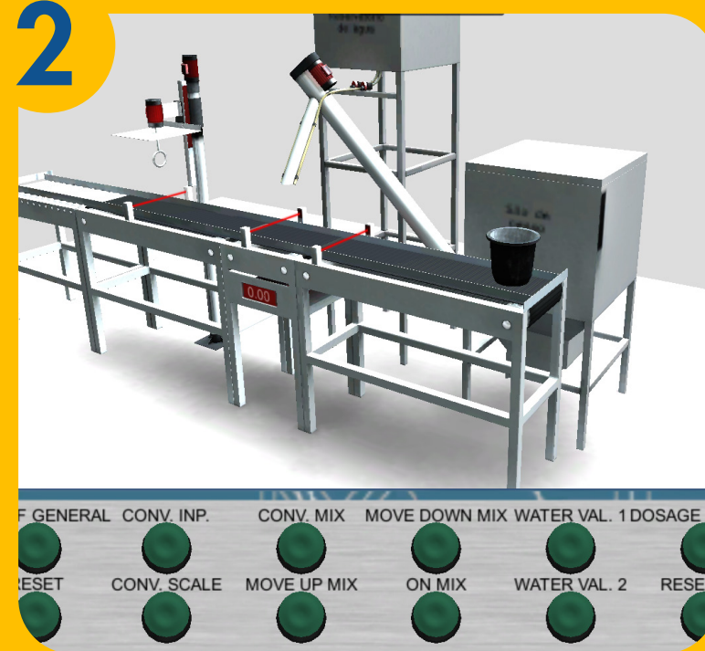
2 GYPSUM DOSING AND MIXING LINE
