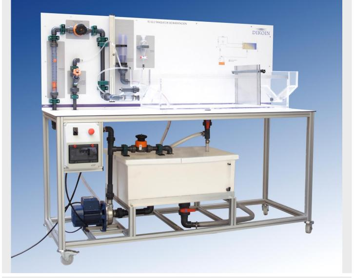
With this equipment is intended to study and visualize in a continuous regime, the natural phenomenon called sedimentation, whereby particles that are denser than the fluid that contains them and in which they are dispersed, fall by gravity depositing in the bottom of the container.
