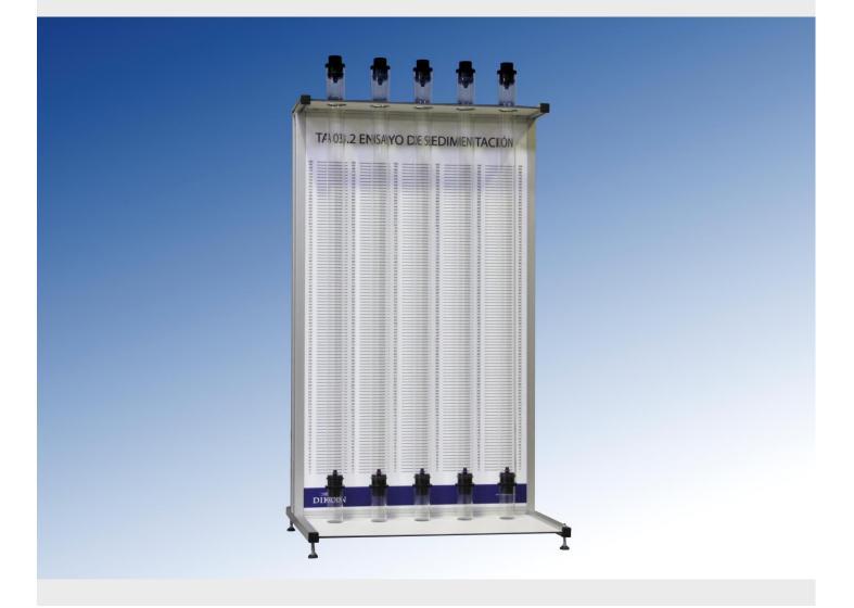
The objective of this equipment is to study and visualize the natural phenomenon called sedimentation, whereby the particles denser than the fluid that contains them and in which they are dispersed, fall by gravity depositing in the bottom.
