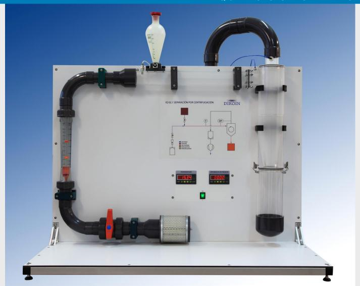
Cyclones are widely used equipment in the industry that allows the separation by centrifugal force of solid particles that are suspended in a gas. They are simple equipments whose operation is based on the separation of the particles by means of the centrifugal force, and that without having movable parts they have a very simple maintenance. As inconvenience we can emphasize that they are not flexible to the changes of concentration, flow or size of the particles.
